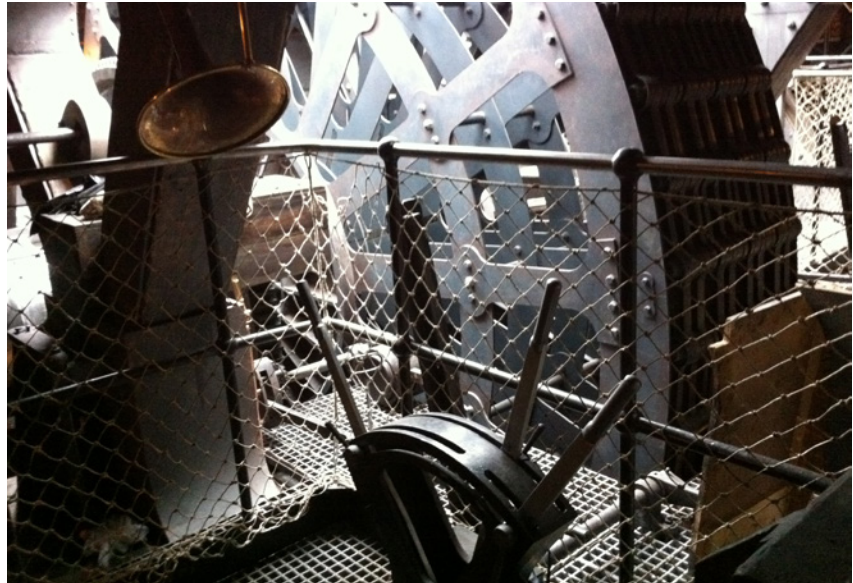
To drive the propeller Brunel designed for ss Great Britain , a massive 1,000hp steam engine. It was the most powerful marine engine of its time. An operating replica of the engine – although not steam driven - has been built for the ship.
